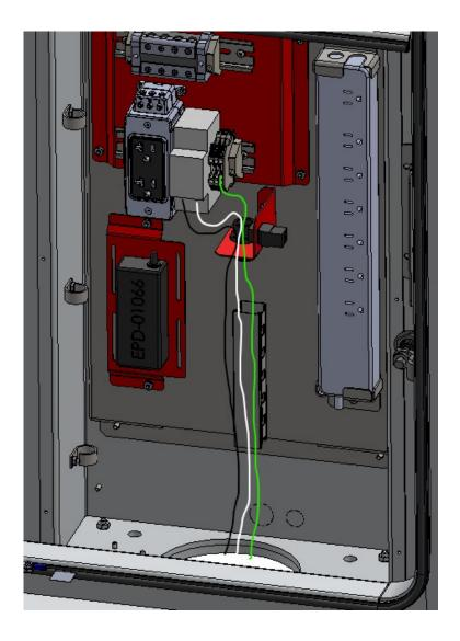
The unit is wired specifically to operate as long as the colored wires coming into and out of the fuse blocks match (white to white and black to black).
